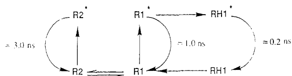
Scheme 1. Proposed model for the fluorescent behaviour of DAPI alone and in complexes with either dsDNA, proteins or phospholipid structures.
